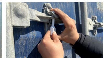
컨테이너 봉인(Seal) 개선(High Security Bolt type)
