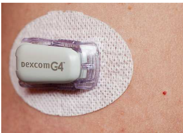
Figure 31. Application of transmitter and sensor Figure 32. Glucose levels monitored via interstitial fluid
